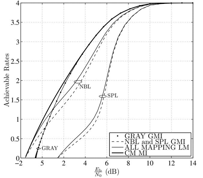
Fig. 1. Comparison of  $I_0(\text{snr})$  and  $I_1(\text{snr})$  for BICM with 16QAM modulation, an AWGN channel and different labelings. The mutual information of CM with 16QAM modulation is also shown for reference.
